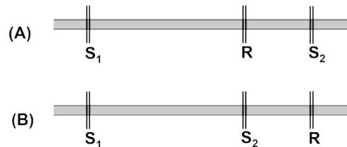
Figure 4.3: (A) Electrode configuration adopted by Gonzalez-Perez et al. Stimulation electrodes are denoted as  $S_1$ ,  $S_2$ , and recording electrodes are denoted as  $R$ . Stimulation electrodes are placed on the two ends of the nerve, recording electrodes are in between two stimulations but close to one side. (B) Electrode configuration adopted by Berg et al. Stimulation electrodes are placed on the same side of the nerve, recording electrodes are at one end of the nerve.
