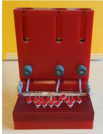
Figure 4.5: A picture of the liquid chamber. On the back are the tubes for injection of solutions, with switches numbered as 1, 2, 3 to control the flow; the glass capillary into which the nerve goes is the transparent cylinder on the base with gold electrodes inside at different positions. The holes in the front are for electrical connections.
