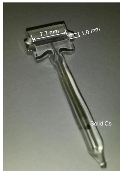
Figure 8.4: A picture of the glass vapor cell. The rectangular channel where the cesium vapor was hold has dimensions of  $1.0 \text{ mm} \times 1.0 \text{ mm} \times 7.7 \text{ mm}$  and is shown on the top of the picture. The channel is connected to a tube with solid cesium via a tiny hole of a micrometer size. The picture is provided by Hans Christian Stærkind from the Quantop group, NBI Copenhagen.
