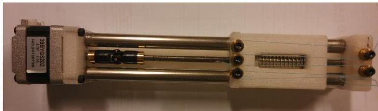
Figure 7.4: A picture of the stretching setup. A bipolar stepper motor on the right side of the picture is attached to a geared track, allowing for stretching when the motor moves.
