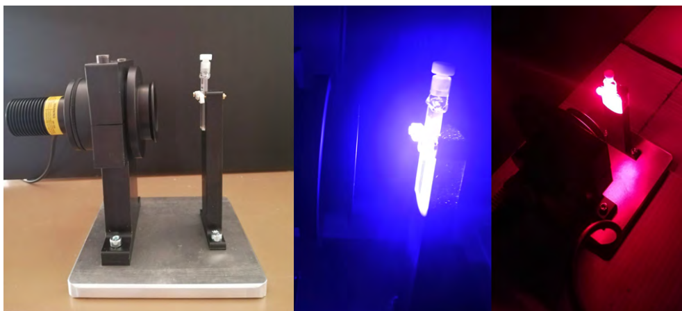
Figure 5.2: On the left, a picture of the homemade irradiation apparatus. On the right, a picture of the set-up with the two different wavelengths LED sources.
