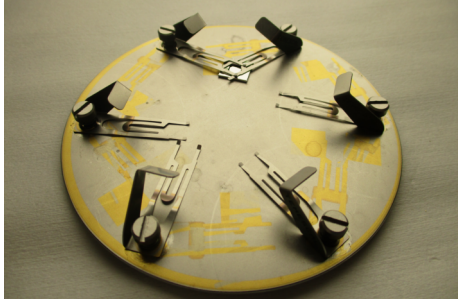
(a) Clamping of one shadow mask and membrane assembly at the upper side of the holder of the e-beam tool.
