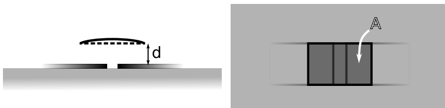
Figure 2.3: Sketch of a parallel plate capacitor, where one plate is mechanically moving. We present a side (left) and top view (right), visualising the relevant geometric parameters, where the extremities fading away lead to the remainder of the circuit.
