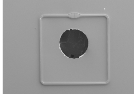
(b) SEM image of the NbTiN loop-gap resonator with etched recess and optics through-hole. The side dimension of the square loop is 1500\ \mu\text{m} and the diameter of the optics hole is \sim 500\ \mu\text{m} .
