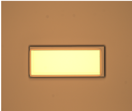
(e) Optical image of the 100\ \mu\text{m} \times 300\ \mu\text{m} , 300\ \text{nm} thick Al spacing pillars used to define the flip-chip distance.
