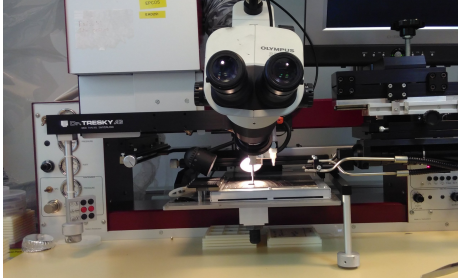
(a) Overview of the flip-chip bonding tool with its microscope, illumination and bottom translation stage.
